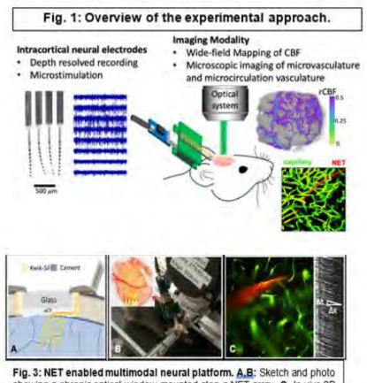
showing a chronic optical window mounted atop a NET array. C, In vivo 2P imaging at 200 µm deep showing the normal density and a intact BBB in the microcapillary (green) surrounding a NET(red). Image taken 2 months after NET implantation. Right: Matrix of line scans showing movement of red blood cells in the capillary marked by the dashed line as dark stripes, the slope of which gives the blood flow speed.
