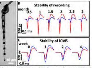
Fig. 2: NET electrodes for stable recording and ICMS. A: Ultraflexible NETs suspended in water where a knot with curvature <50 µm was made. B: Chronically stable recording of a single-unit action potential over 3 months. C: ICMS that repeatedly activated the same units (red and blue) for 4 weeks.
